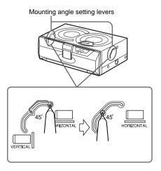
Insert a pointed object such as a screw driver or ball-point pen, etc. into the low spot of the lever and slide the lever to the position from among HORIZONTAL, 45°, and VERTICAL positions.
